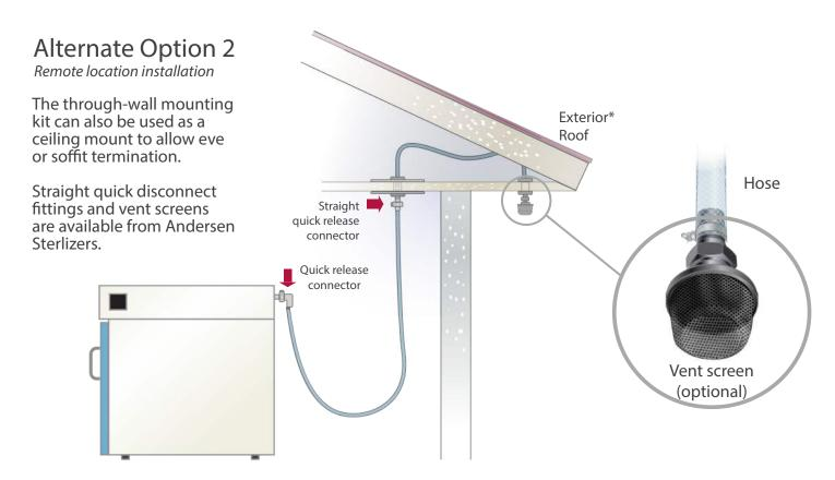
Important: Each EOGas 4 Sterilizer must have its own dedicated exhaust to outside air. The exhaust streams from multiple sterilizers may <u>not</u> be combined into a single exhaust stream that then vents to the outside.
