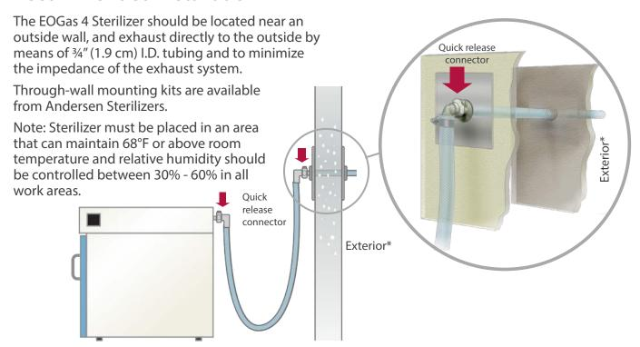
The EOGas 4 Sterilizer must be installed adjacent to an unswitched, non-GFCI, grounded power outlet that is dedicated to its exclusive use.
