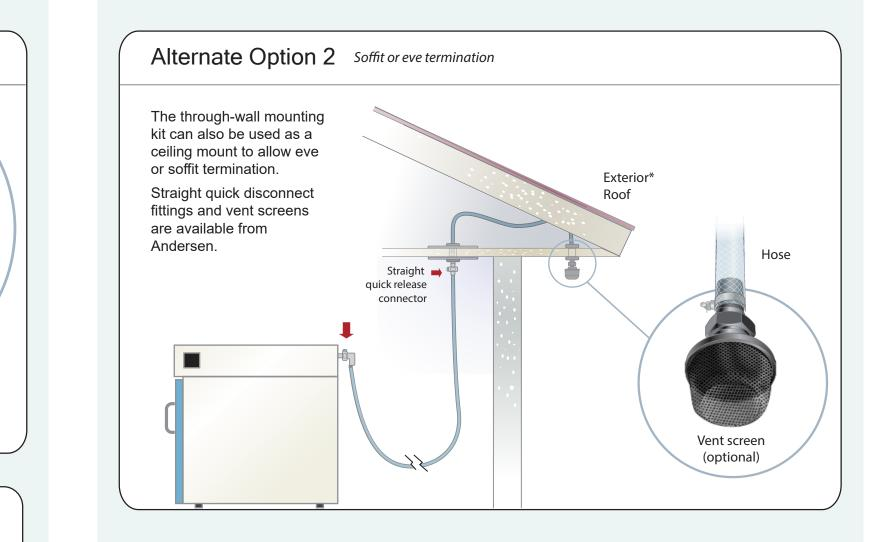
\* Please note: AAMI guidelines recommend all EO sterilizers be vented through a dedicated exhaut line to the outside atmosphere directly or through an emission control system. The vent should not terminate within 25 feet of any building air intake source or near pedestrian or animal traffic, nor should it allow EO release into or to reenter the building.
