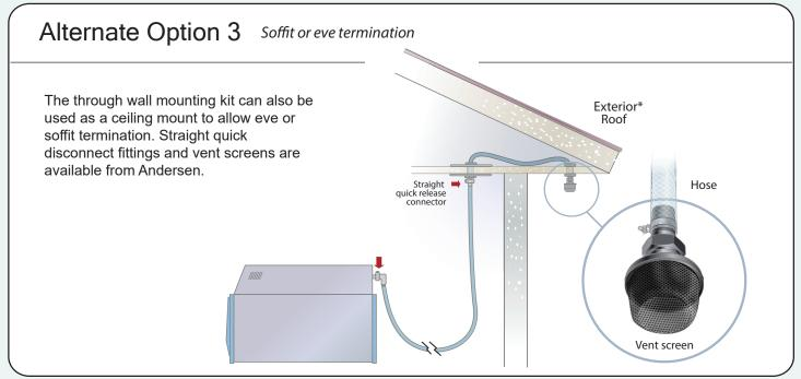
\* Please note: AAMI guidelines recommend all EO sterilizers be vented through a dedicated exhaut line to the outside atmosphere directly or through an emission control system. The vent should not terminate within 25 feet of any building air intake source or near pedestrian or animal traffic, nor should it allow EO release into or to reenter the building.
