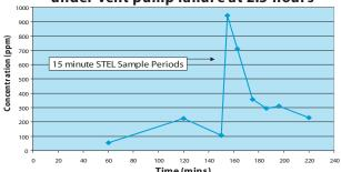
A gas chromatograph (GC) was used to test the concentration of ethylene oxide in the air samples.
