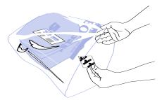
Remove an EOGas cartridge from the dispenser box. Confirm that the number printed on the EOGas cartridge corresponds with the number printed on the sterilization bag. Remove the trigger guard (secured with green tape) and place the EOGas cartridge on top of the devices near the open end of the sterilization bag in a horizontal orientation (long edge of cartridge as parallel to the floor as possible), but **do not activate the cartridge at this time.**
