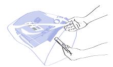
Remove excess air with a vacuum sealer or press the excess air out of the sterilization bag before heat sealing, then initiate the sterilization cycle by pressing the LOAD key on the front of the EOGas sterilizer cabinet and follow the directions for loading.
