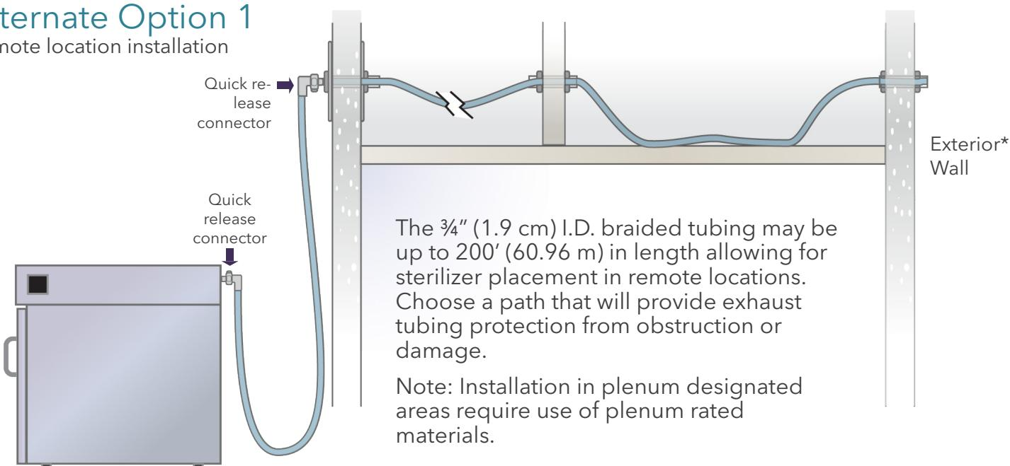
The  $\frac{3}{4}$ " (1.9 cm) I.D. braided tubing may be up to 200' (60.96 m) in length allowing for sterilizer placement in remote locations. Choose a path that will provide exhaust tubing protection from obstruction or damage.
