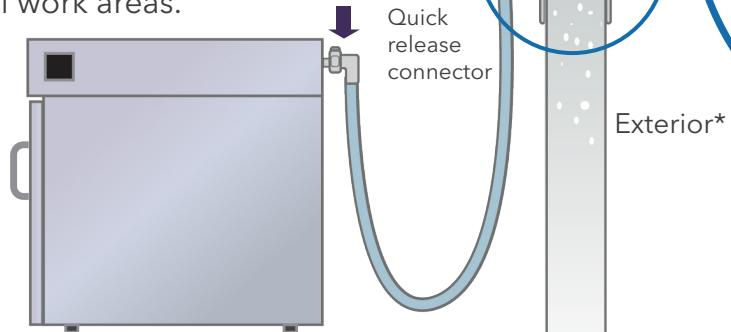
The EO<sup>+</sup>Gas 4<sup>PLUS</sup> Sterilizer must be installed adjacent to an unswitched, non-GFCI, grounded power outlet that is dedicated to its exclusive use.
