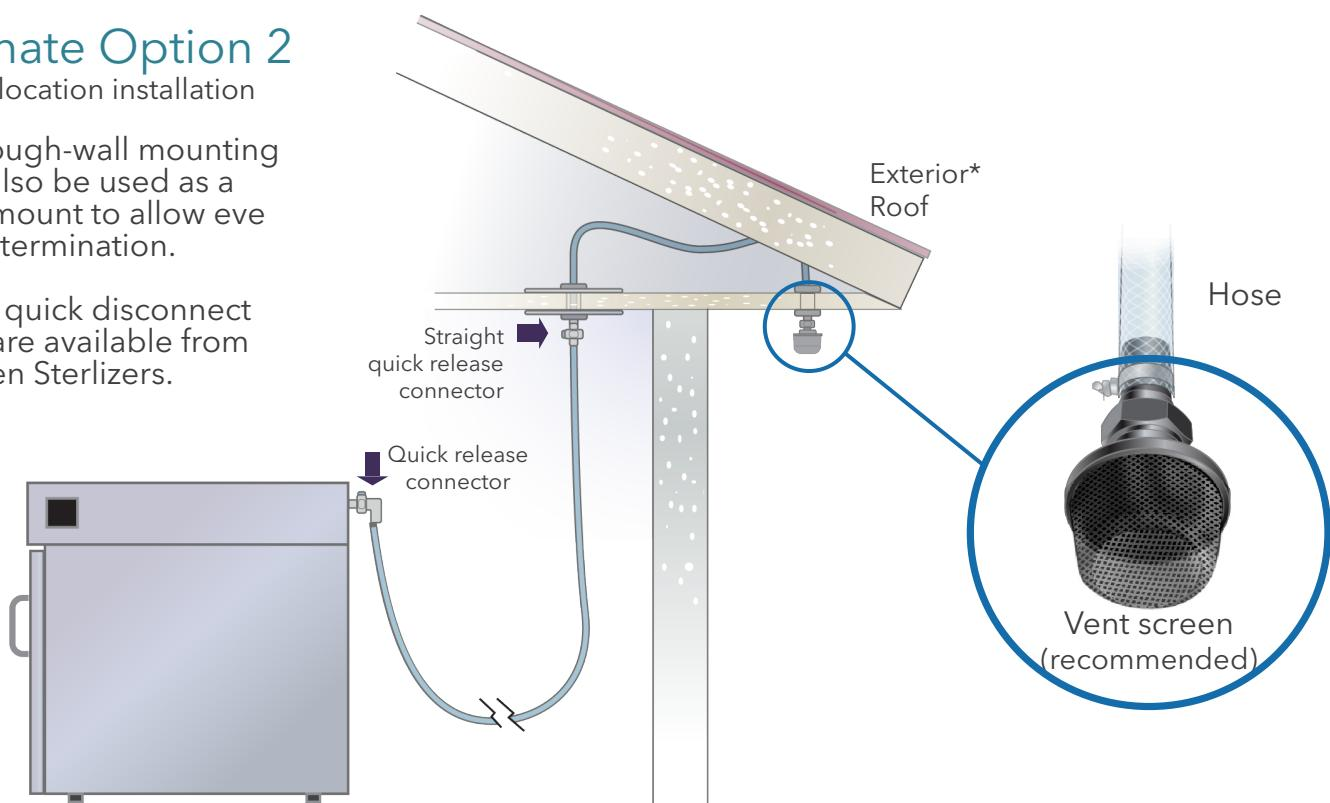
**Important:** Each EO Gas 4<sup>PLUS</sup> Sterilizer must have its own dedicated exhaust to outside air. The exhaust streams from multiple sterilizers may not be combined into a single exhaust stream that then vents to the outside.
