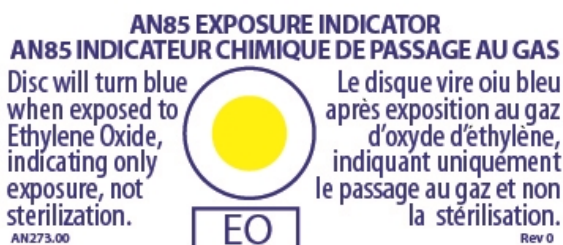
Indicator label prior to Ethylene Oxide Exposure
