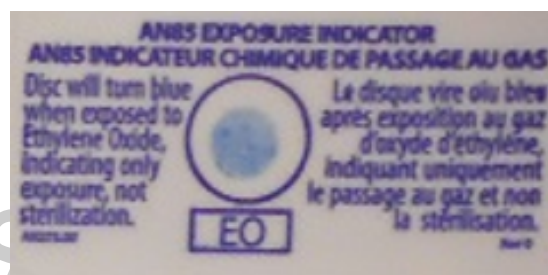
Indicator label after Ethylene Oxide Exposure
