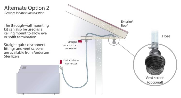
Important: Do not combine the exhausts from multiple units into a single exhaust stream as this will adversely affect the safety and performance of the sterilizer.
