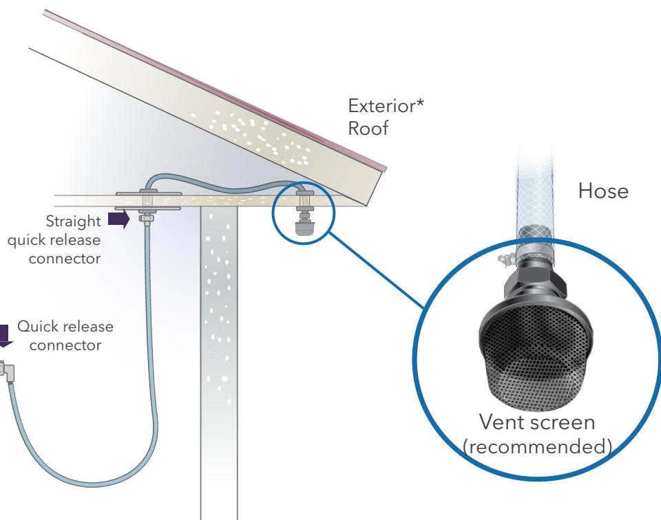
**Important:** Do not combine the exhausts from multiple units into a single exhaust stream as this will adversely affect the safety and performance of the sterilizer.
