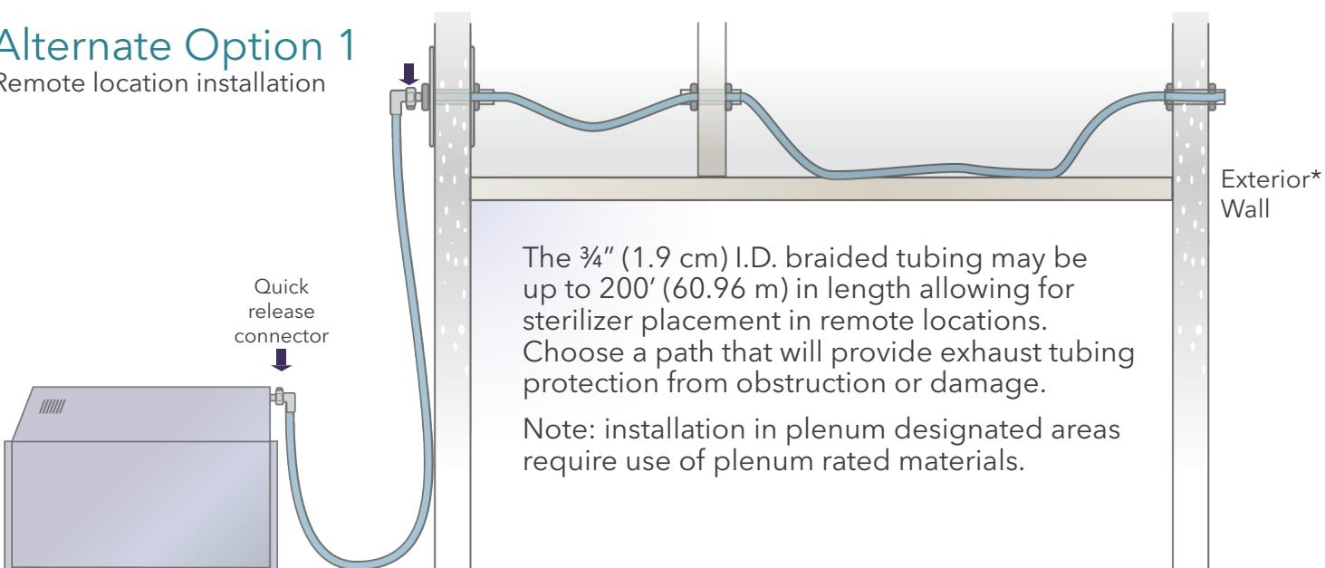
The  $\frac{3}{4}$ " (1.9 cm) I.D. braided tubing may be up to 200' (60.96 m) in length allowing for sterilizer placement in remote locations.
